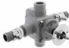
Pressure balance valve less diverter - 1/2" rough valve only. Flow rate 7 GPM @ 50 PSI.
