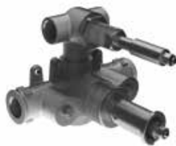
5 5/16" (135mm) 5 5/16" (130mm) 1/2" thermostatic rough-in valve only with integral two port non-sharing diverter and shut-off 5.5 gpm (gallons per minute) flow rate (@60 psi)
