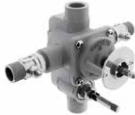
Pressure balance valve with diverter - 1/2" rough valve only. Flow rate 7 GPM @ 50 PSI.
